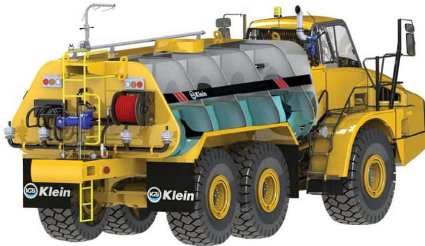
Throughout history, the design of the mobile truck tank has evolved. Evolving designs have improved strength, maximized payload efficiency and enhanced job site and operator safety. Klein Products has provided leadership, innovation and design achievement since the 1950's. The standard tank shape design in the early years was a simple, cost-effective "round" tank design, which then led to an "oval" design. These shapes were then typical of all mobile tank manufacturers.
